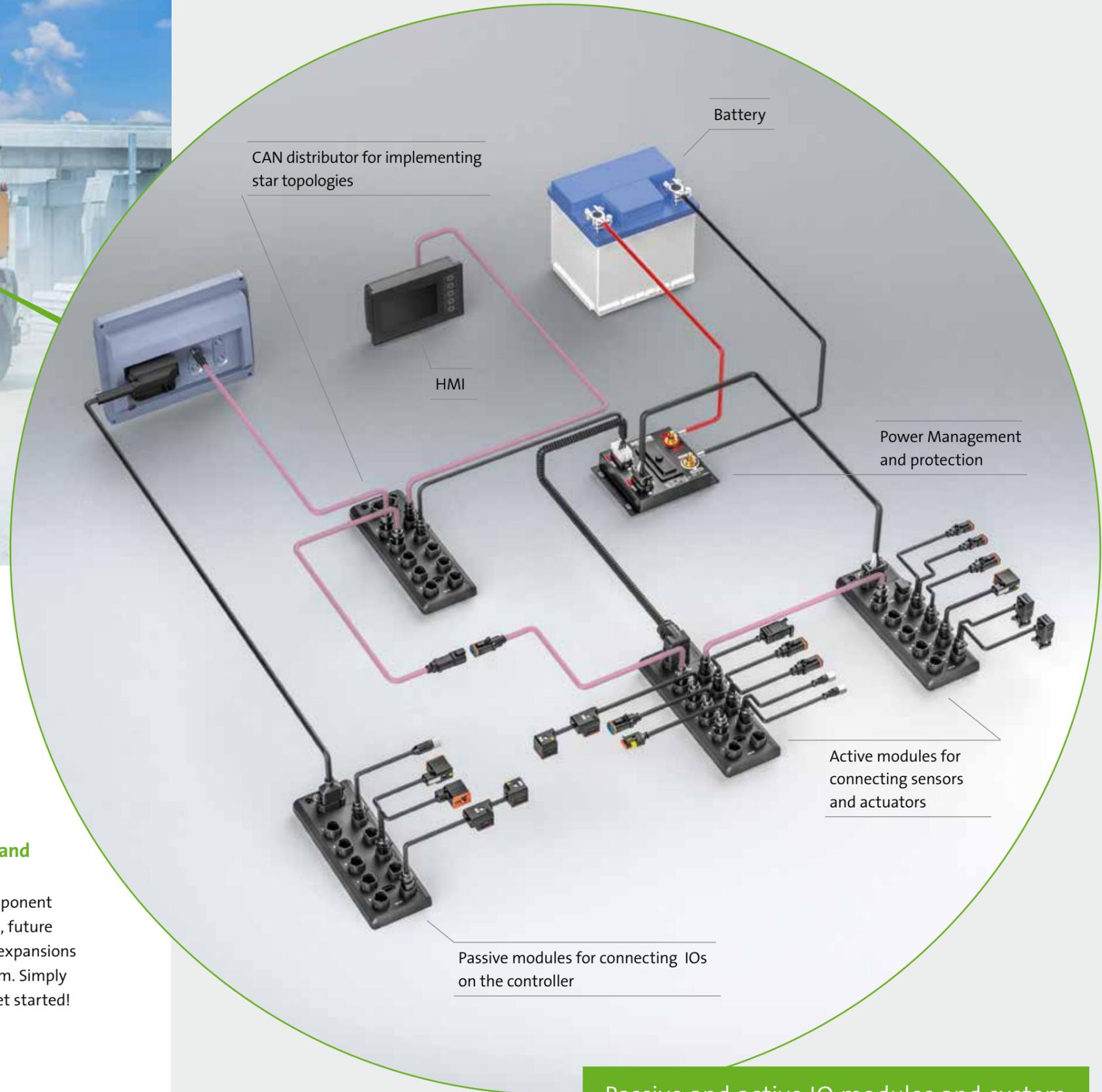
With Murrelektronik and Data Panel's modular installation system you can easily solve IO installation challenges in mobile machines
